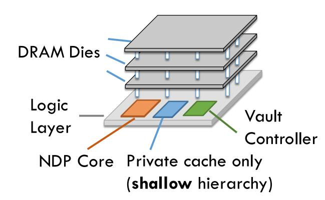
Conventional multicore processors use a multi-level **deep** cache hierarchy to reduce data movement
