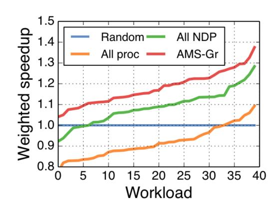
Always processor never leverages the NDP capability of the asymmetric system and is 8% worse than Random
