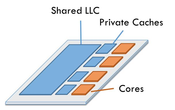
Conventional multicore processors use a multi-level **deep** cache hierarchy to reduce data movement
